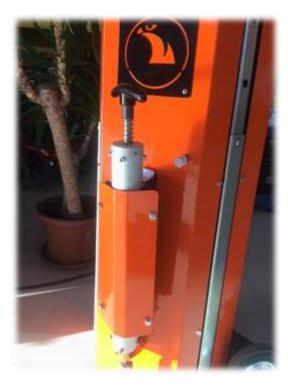
EASY pneumatic air pump with air valve to release the mast
